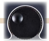
The round **zoom wheel** is in the middle of the control panel. This zoom wheel controls magnification for the text and other items viewed with your **VisioBook**. Turn the wheel clockwise to increase magnification. Turn it counterclockwise to decrease magnification.
