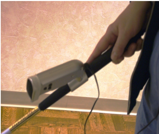
Figure 17: Alternate Grip Becomes Unbalanced When Hand is Behind the 'K' Sonar
