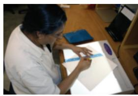
There are many different ways to create tactile graphics. At the left, a transcriber works with a spur wheel to produces lines with raised dots. She will heat the master graphic in the thermoform machine (rear of photo) to create plastic copies that will be included in textbooks. At the right, a tactile graphics producer uses background lighting from a light box to draw lines on a graphic. The center photo shows collage graphic supplies and tactile graphics being developed.
